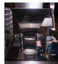
Integration Chute enters bag to prevent spillage and protect seal area
